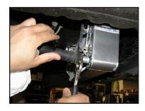
12. COOLANT ALERT!!!!! Remove the pump inlet hose and rotate the pump so the outlet points toward the rear and slightly upward. Coolant will come out of the pump unless you rotate the outlet over the top. Also, you may want to shift the pump 1" to the driver's side. This is done to give a little extra clearance on the hose. Tighten the two bolts on the clamp that secure the pump. Reconnect the inlet hose to the pump and install the clamp.
