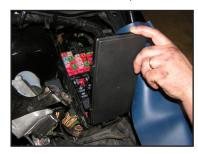
28. Remove the plastic loom on the coolant pump harness at the connecter and locate the white wire on the harness. This wire may be a different color, but you need the wire that is in the #2 pin location. This wire will have battery voltage when pump is activated. Cut this wire approximately 2" from the pump connecter.
