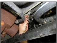
33. Reconnect the coolant pump connecter and resistor connecter.
