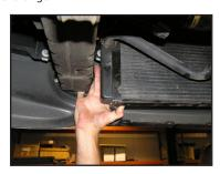
9. Install the aluminum upper bracket and attach using the two factory bolts in the factory holes. Use the two 1/2" long button head bolts and flange nuts supplied in the kit in the front holes. The spread on the OE heat exchanger brackets vary from vehicle to vehicle. They can be easily moved by hand. Tighten the bolts.
