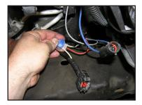
30. Run the harness back over the frame rail and fasten to keep out any slack in the harness in the areas of engine compartment and in front of the tire.
