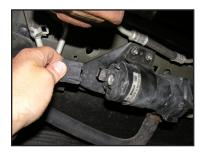
Loosen the two bolts on the clamp securing the coolant pump and rotate upward to lessen the chance of coolant running out.
