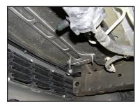
Install the AFCO HEAT EXCHANGER to the upper bracket and install the four washers and serrated nuts. Tighten the nuts.
