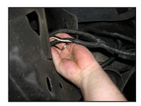
31. Connect the two weatherpack connecters to the connecters on the fans. The longest section connects to the passenger side fan and the shortest section connects to the driver side fan.
