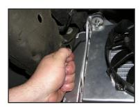
17. Disconnect the MAF(Mass Air Flow) sensor.
