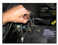
Remove the rubber filler between the valance and the lower heat exchanger bracket. This will be reused if you have the fan and shroud kit.
