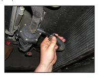
6. Disconnect the coolant pump harness and the resistor connecter above the pump.
