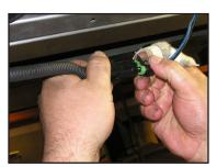
32. Remove the driver side bolt on the coolant pump bracket. Attach the terminals on the black & grey fan harness ground wires to this location and reinstall holt
