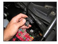
25. Run the harness along side the fuse box and push the retainer installed in step 22 into the predrilled hole in the inner fender.
