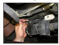
8. Remove the two bolts securing the lower heat exchanger bracket to the bumper bracket. Save these bolts-You will reuse them. NOTE - The lower bracket has two "J" hooks on the front. Swing the heat exchanger down and forward and remove the upper rubber saddles. This will allow you to push the heat exchanger up to unhook the brackets. Remove the lower bracket and heat exchanger.
