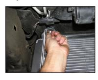
Attach the lower hose to the lower fitting of the AFCO Heat Exchanger and install the hose clamp.
