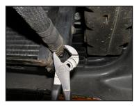
Disconnect the upper hose from the coolant pump.
