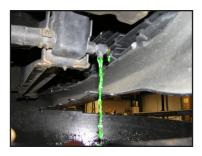
Disconnect the lower hose from the factory heat exchanger.
