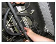
14. Route the hose as shown and attach the other end to the AFCO HEAT EXCHANGER and install the supplied clamp.
