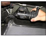
Attach one end of the piece of straight hose supplied with the kit to the pump outlet and install the supplied clamp.
